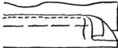
Lapped or tucked seam
